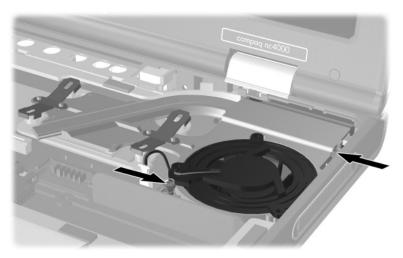
Spring-Loaded Torx T8 M2.0×10.0 Screw Locations
